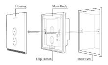
3. Close the housing to finish installation (Join the network before closing the housing).
